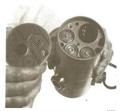
Fig. 6 Inserting batteries
